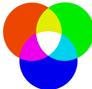
Fig. 2. Equal amounts of light from overlapping red, green, and blue spotlights produce white.
